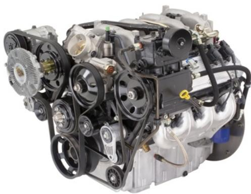
The compression ratio on this generation of engine was typically 9.1:1, and HP up to 330 HP and 450 ft. lbs. of torque. Unique to the Vortec 8100 over many contemporary engines is its returnless fuel system with anti-reflux valve. GM equipped vehicles of this engine can include the 2500HD / 3500 series trucks, including the Avalanche, Silverado, Suburban, Sierra, Yukon XL, up into the medium duty trucks like the Kodiak, TopKick and Workhorse.
