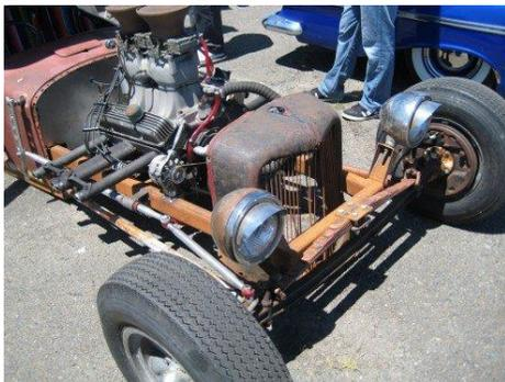
"Junk yard parts and ingenuity are the staples of rat rods. If you look close, you can see the suspension on this vehicle is composed of an inverted leaf spring bolted to the chassis by a square plate& mash; hardly high tech!"
